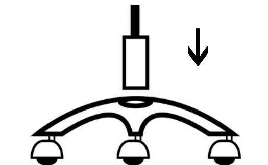
On the floor, insert cylinder into arm base and press.
