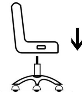
Cylinder insert into the hole at the bottom of seat.
